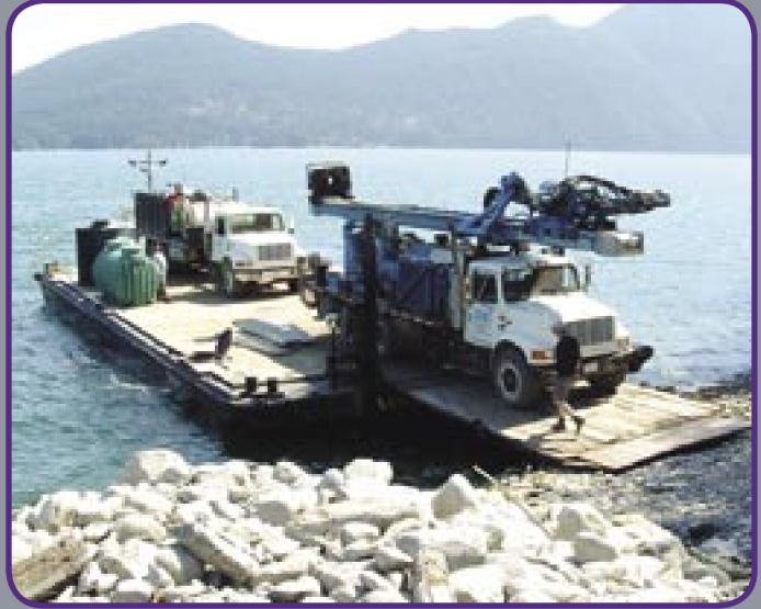
■ Preparations for over water sampling program for earth dam investigation.
