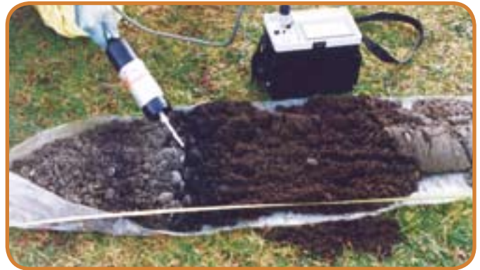
■ Field testing with a gas detector
