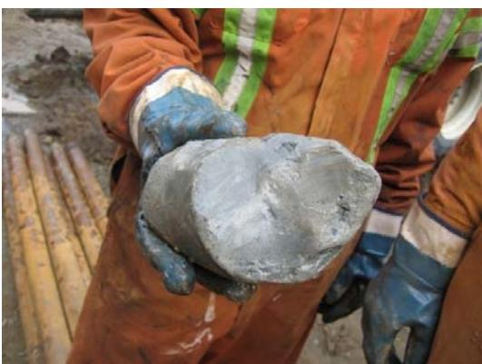
With a small working space, a tight budget, and silty, sandy ground beneath them, the Magees arranged for a sonic drill rig to bore four holes, each to a depth of 200 ft.
